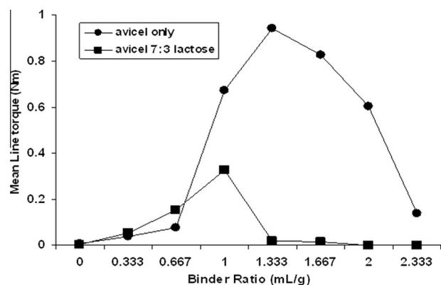
**Figure 5** Mean torque for Avicel® PH101 and Avicel® PH101-lactose (7:3) mixture using water as a binder.
