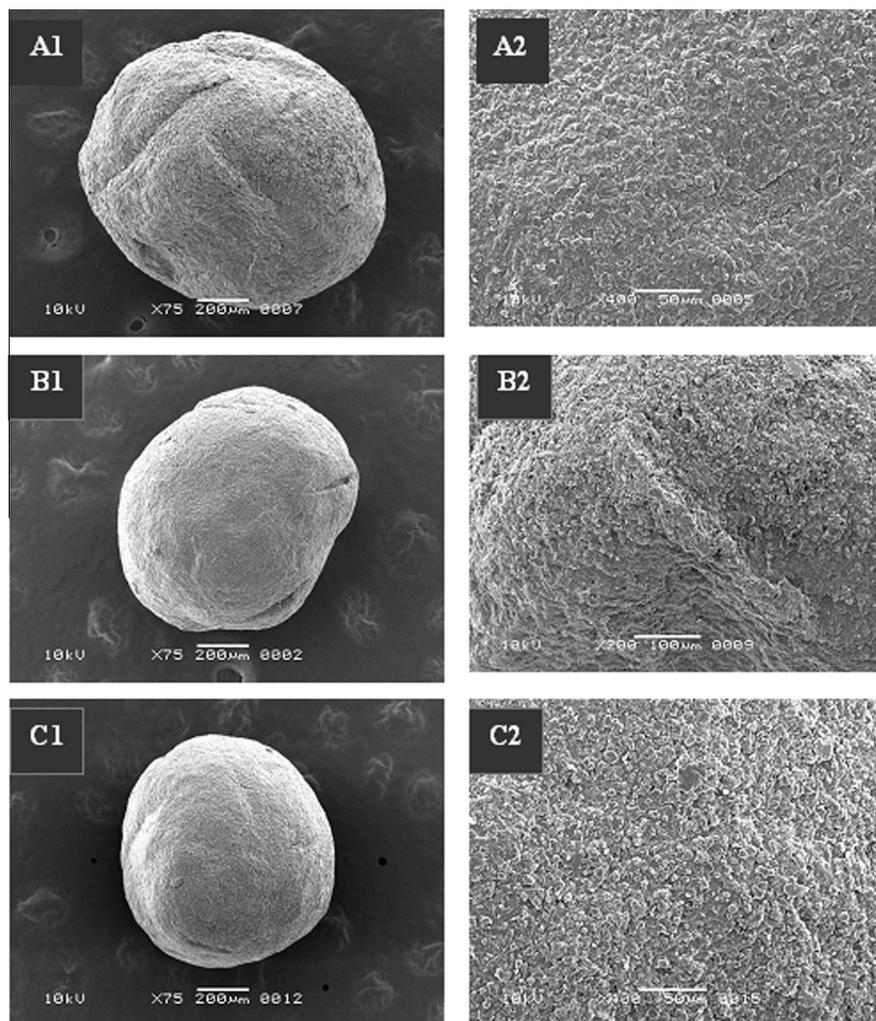
**Figure 6** (A) Scanning electron micrographs of pellets containing untreated FM, (B) pellets containing FM-Pluronic (1:3) solid dispersion and (C) pellets containing FM-Gelucire (1:3) solid dispersion.
