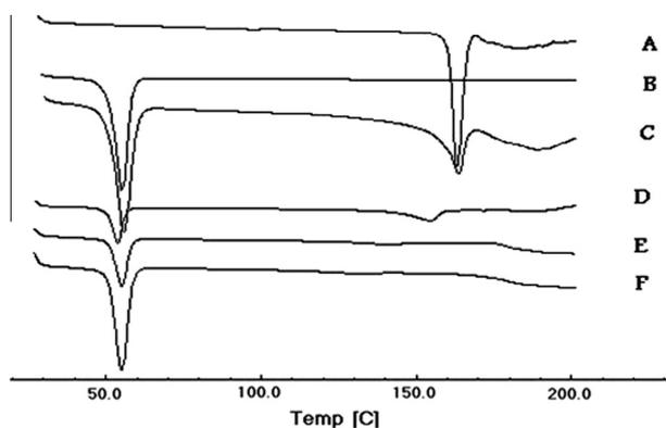
**Figure 2** DSC curves of FM (A), Pluronic (B), FM-Pluronic (1:3) physical mixture (C), FM-Pluronic (1:1) solid dispersion (D), FM-Pluronic (1:3) solid dispersion (E) and FM-Pluronic (1:5) solid dispersion (F).
