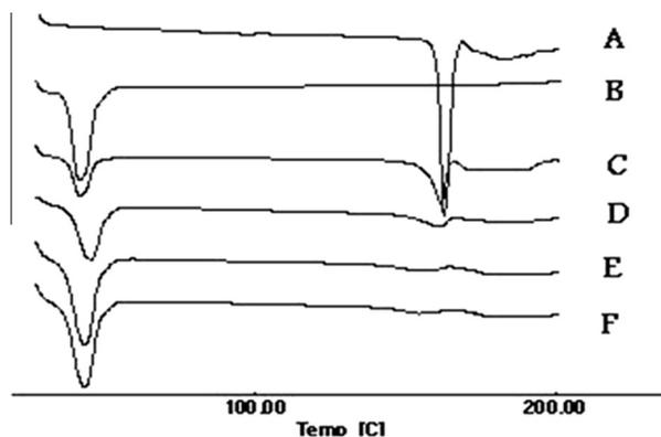
**Figure 1** DSC curves of FM (A), Gelucire 50/30 (B), FM-Gelucire (1:3) physical mixture (C), FM-Gelucire (1:1) solid dispersion (D), FM-Gelucire (1:3) solid dispersion (E) and FM-Gelucire (1:5) solid dispersion (F).
