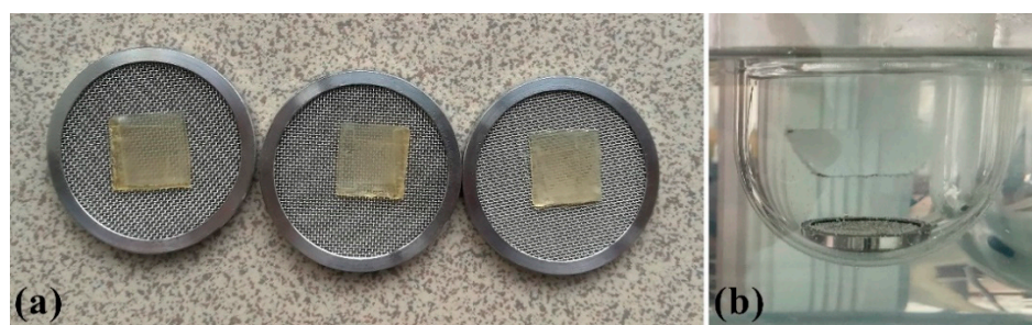
Figure 3. (a) Samples on metal mesh disc; (b) set up for dissolution test.
