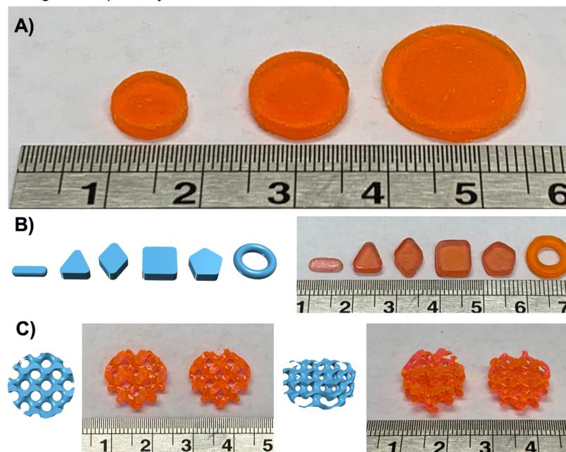
Figure 3. A) Photographs of (from left to right) size-8, size-11, and size-16 Printlets; 3D models (left) and photographs (right) of B) Printlets in various geometries, and C) gyroid lattice Printlets. Scale shown in cm.
