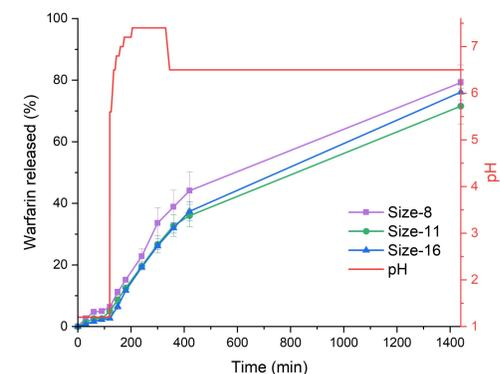
Figure 5. Cumulative release profiles of EOS2 size-8, size-11, and size-16 Printlets. Data values represent mean  $\pm$  SD (n=3).
