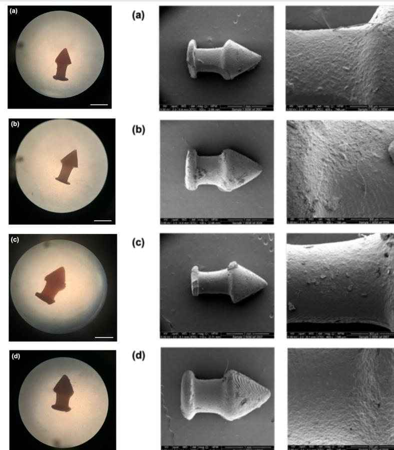
**Figure 3.** Light microscope images (left) and SEM images (right) of the DLP 3D printed (a) D10, (b) D10PEG, (c) D20, and (d) D20PEG punctal plugs. The scale bar is equivalent to 1mm.
