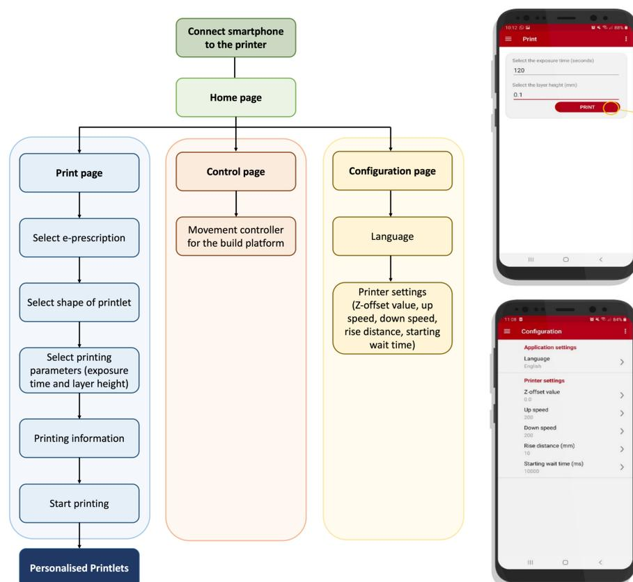
Figure 2. Flow chart of a smartphone-enabled 3D printing process using the custom mobile printing app
