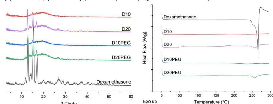
**Figure 4.** X-ray powder diffraction patterns (left) and DSC scans (right) of dexamethasone and DLP 3D printed formulations.
