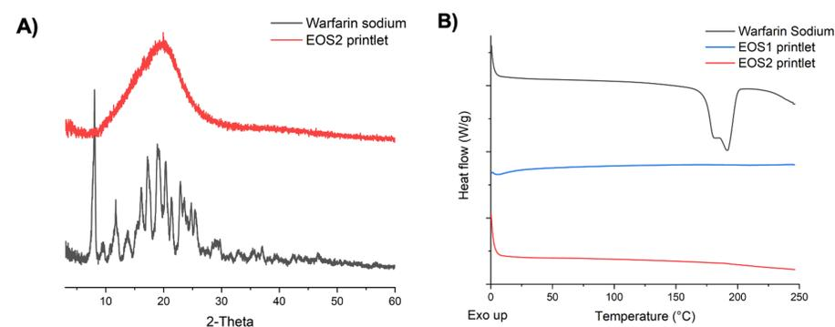
Figure 4. A) X-ray powder diffractograms, and B) DSC thermograms of warfarin, EOS1 Printlet, and EOS2 Printlet.
