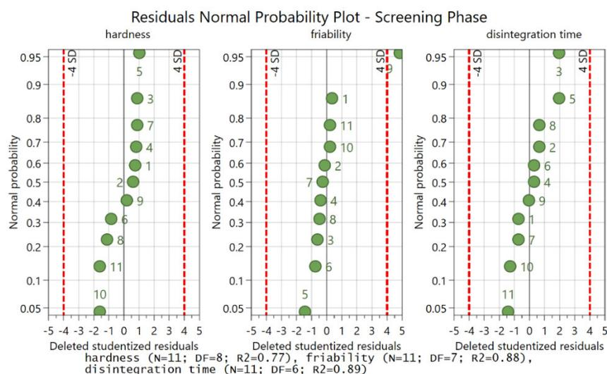
**Figure A2.** Normal probability plot showing the normal distribution of results for hardness, friability, and disintegration time of tablets during the screening phase of the DoE study.
