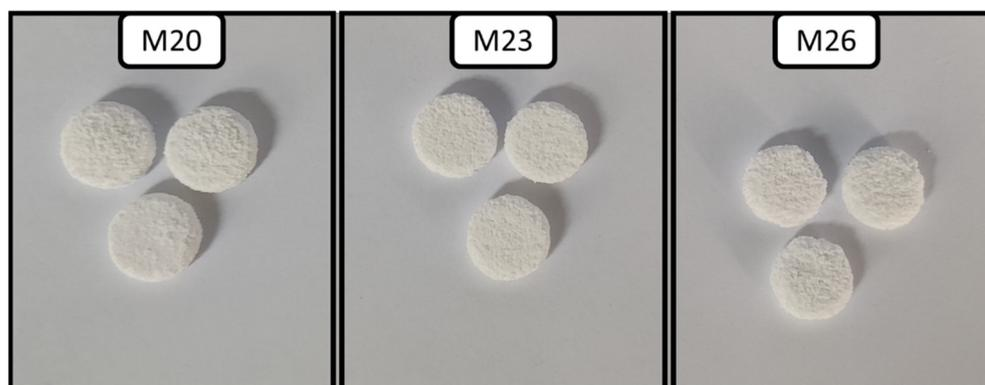
**Figure A1.** Visual representation of 3D-printed tablets from experiments M20 (high strength), M23 (medium strength), and M26 (low strength) with the 20% ethanol-water mixture. As can be discerned, an excess of material at tablet edges is observed for experiment M20, while experiment M26 yielded poorly bonded tablets due to high layer height and low saturation.
