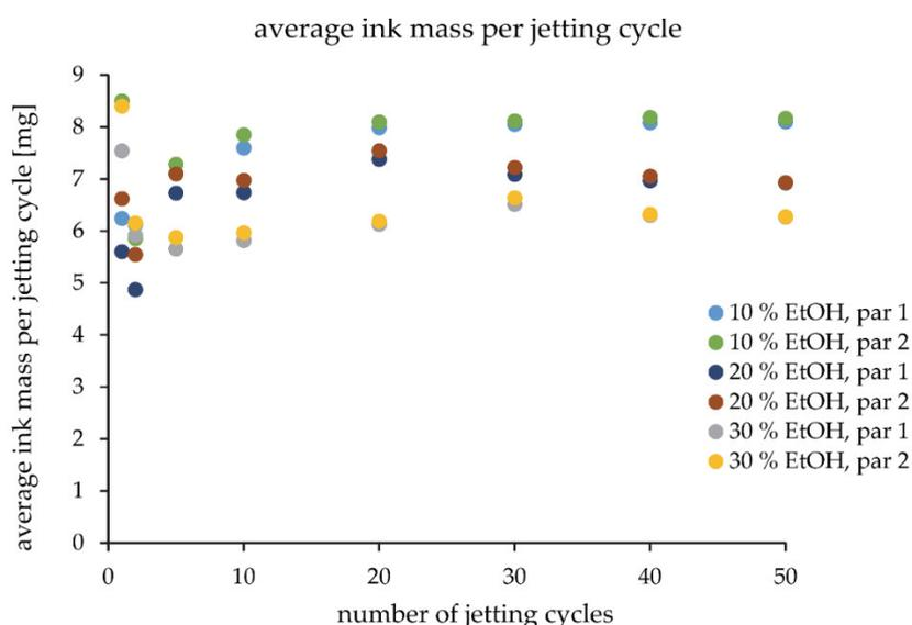
**Figure 5.** Average ink mass per jetting cycle over many layers. Par 1 and par 2 denote two parallel experiments to check for repeatability of measurements.
