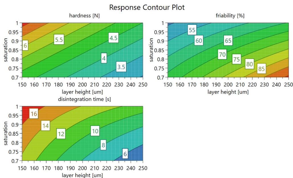
**Figure 3.** Response contour plot revealing the influence of layer height and the saturation parameter on the mechanical properties of tablets.
