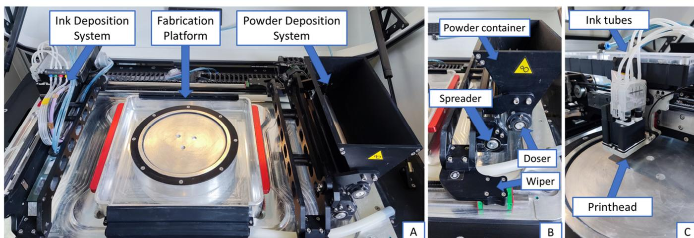
**Figure 1.** Key components of the Picojet D220 3D printer. The main parts are displayed in (A), the powder deposition system in (B) and the ink deposition system in (C).
