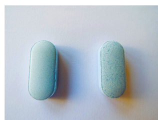
Figure 4: Tablets made with PROSOLV® SMCC versus microcrystalline cellulose and colloidal silicon dioxide.
