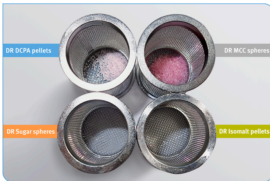
Fig. 7. Residues of diclofenac sodium DR pellets (DCPA, MCC, sugar, isomalt) at the bottom of basket after completing the buffer stage.
