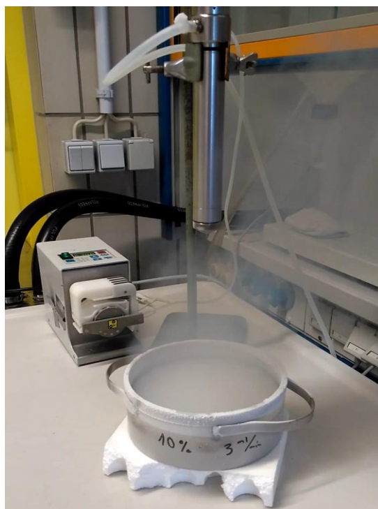
Figure 23: Schematic overview of lab scale SFD apparatus.
