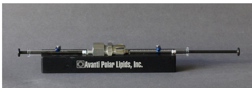
Figure 20: Avanti Mini-Extruder constructed of stainless steel and Teflon. Two polycarbonate membranes and filter supports are placed between two Teflon bearings and membrane supports. The heating block allows the extrusion of vesicles for lipids which have a transition temperature above room temperature.
