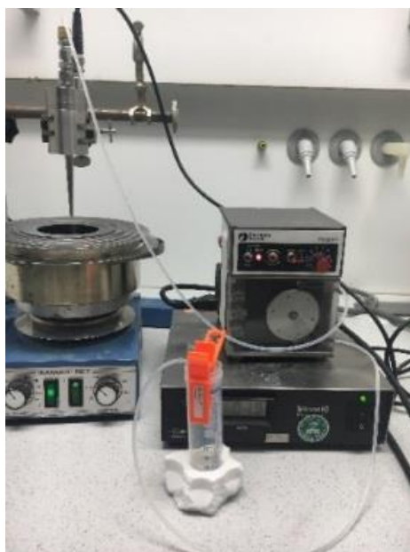
Figure 22: Experimental setup of proliposomal production in small scale.
