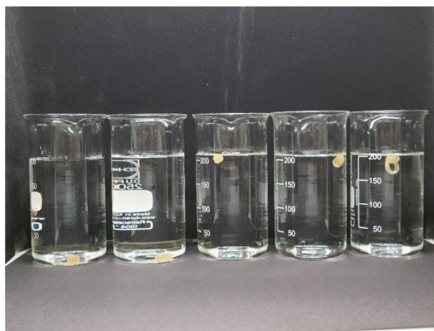
Figure 7. Floating comparison of cylinder, D12, float, cylinder–float (CF) and ring–float (RF) solid dosage forms from left.
