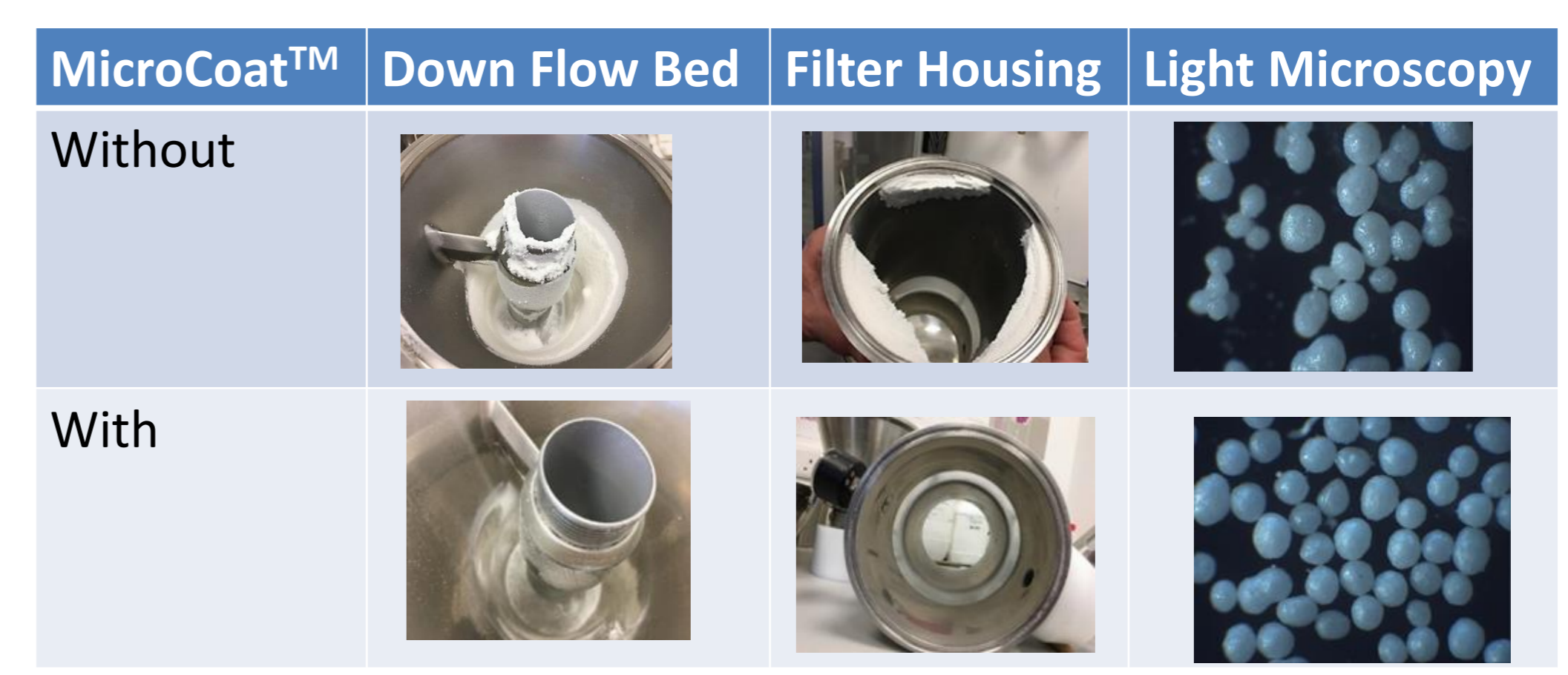
Figure 1. Equipment appearance and light microscopy of coated microparticles following coating without (top) and with (bottom) MicroCoat™ technology
