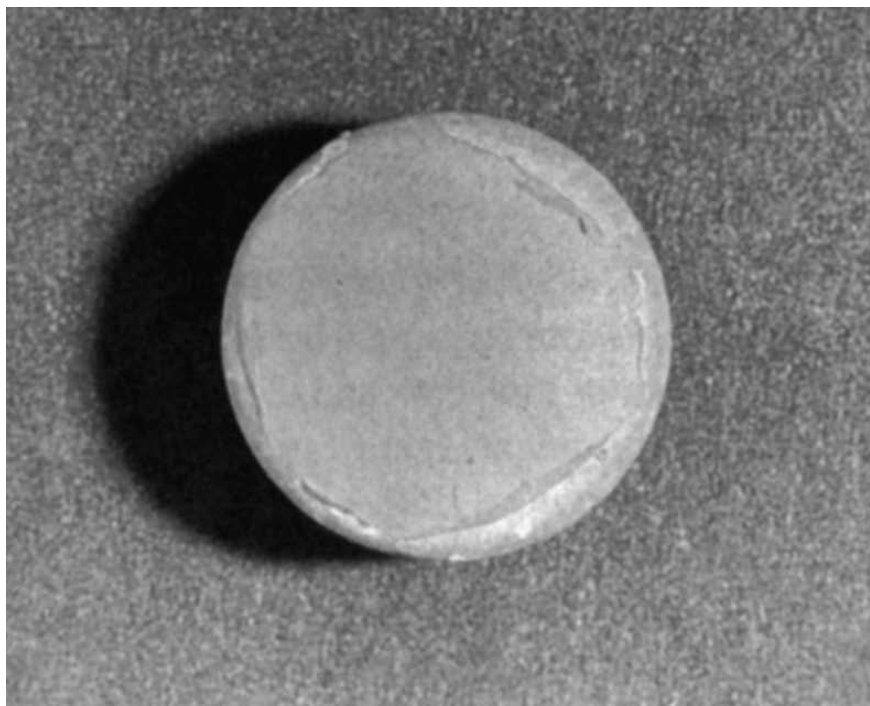
Fig. 90: Peeling and flaking at the edge of the tablet
