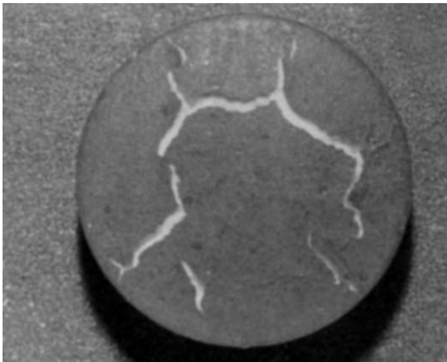
Fig. 89: Cracking and splitting on the tablet surface
