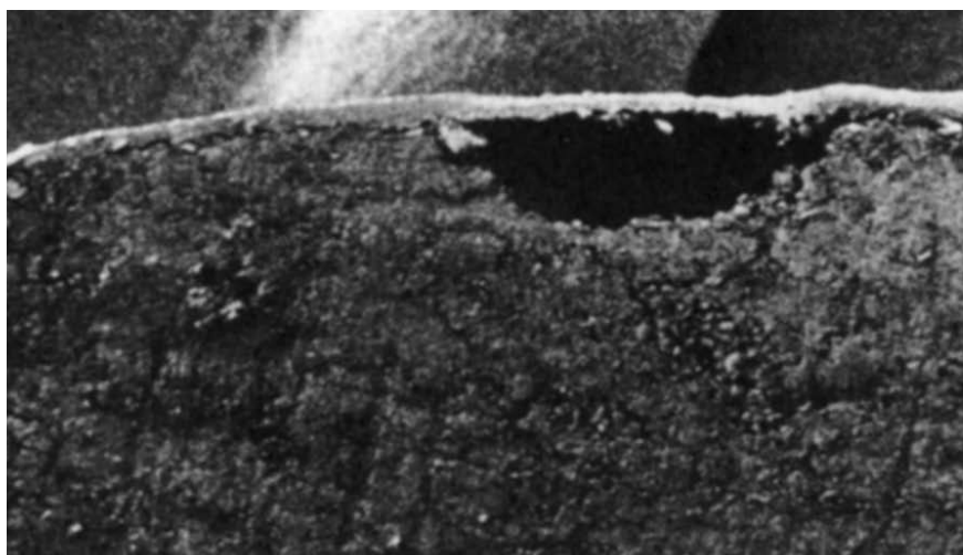
Fig. 91: Bridging effect (cross-section of a tablet)
