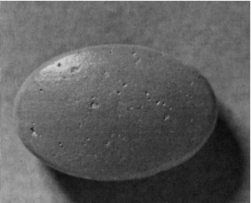
Fig. 92: Pitting in the film caused by stearic acid
