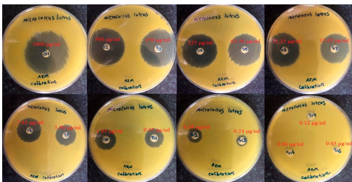
Figure 7. Zone of growth inhibition by Micrococcus luteus in the analysis of azithromycin.
