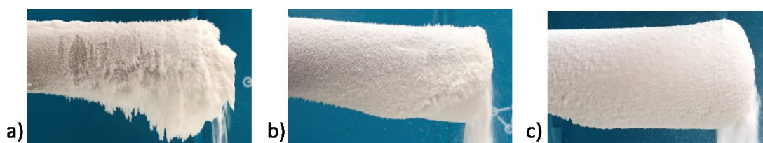
Figure 21 Examples of electrostatic powder buildup of HPMC K4M CR at feed rates of a) 1 kg/h; b) 7.5 kg/h; c) 15 kg/h
