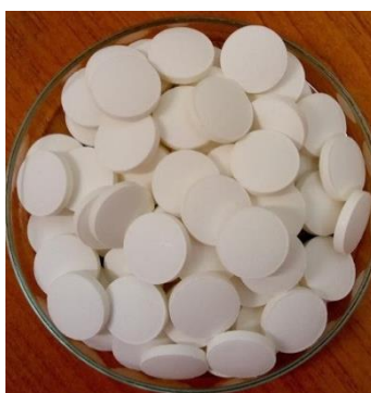
Figure 24 Tablets prepared from ground fibrous enzyme-containing powder, MCC, mannitol, croscarmellose sodium, and magnesium stearate
