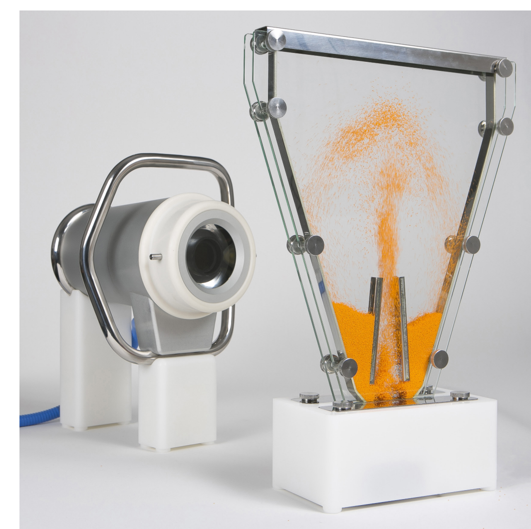
Figure 1: Image acquisition of pellets in a 2D fluid-bed system (right) with visual inspection system PATVIS APA (left).
