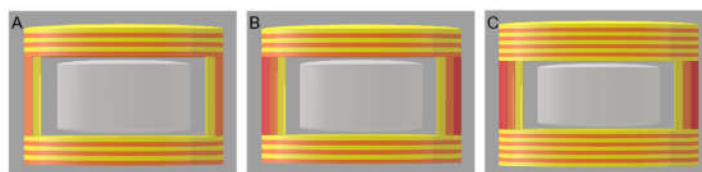
Figure 2. 3D-printed tablets with different thicknesses of outer shell: (A) FH-95-266, (B) FH-95-366, (C) FH-95-399.
