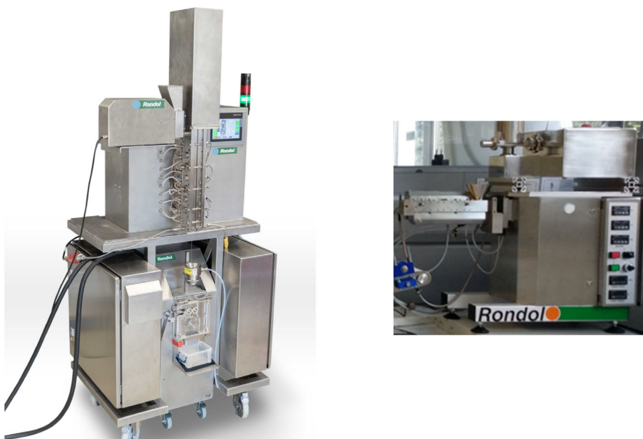
FIGURE 1 Vertical all in one extruder twin screw 10 mm 40/1 D (left) and horizontal twin screw 10 mm 20/1 D (right) RONDOL Industrie
