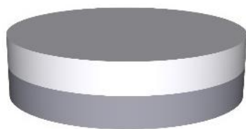
Figure 2. 3D visual design of overprinting tablet: diameter: 10 mm; top layer overprinted thickness: 1.8 mm; and bottom layer injection molded thickness: 1.8 mm.
