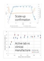
At pilot scale the granule moisture tends to decrease with the EE/DC ratio equal to 100% (scale difference). The process model was improved to better describe the pilot scale process, and the drying model Burgschweiger and Tsotsas [4] with an additional evaporation term was used.
