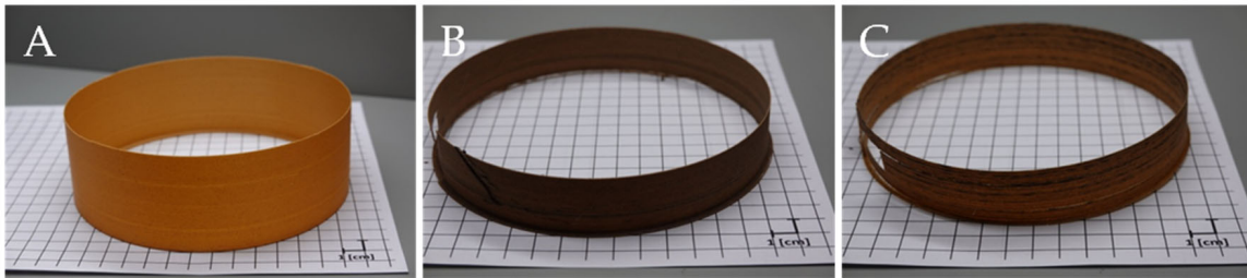
Figure 11. L-FDM-printed cylinders of PLA WOOD (A–C) modified with: (A) reference sample not modified marked ref. 6, (B) silver nitrate marked 6.4, and (C) iron (III) chloride marked 6.5.
