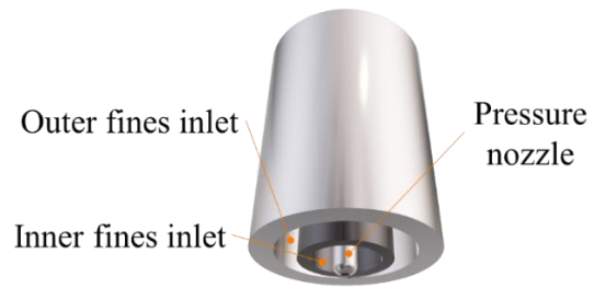
Figure 2: Schematic overview of the nozzle and inlet position of the fines, not to scale. Also pictured is the 25 cm extension of the inner/outer tubes.
