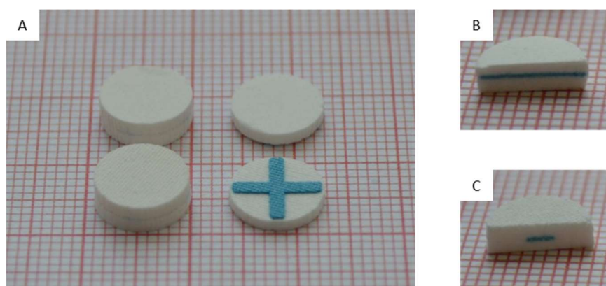
Figure 4. Photographs of 3D screen-printed tablets in disk-shape on millimeter paper. Finished tablet and demonstration tablet with a blue cross (A), tablet with an anti-counterfeiting marker broken exactly in the middle (B) or slightly off-center (C) reveals the respective parts of the blue cross.
