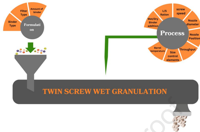
Figure 27: Schematic Diagram of Twin screw wet granulation.
