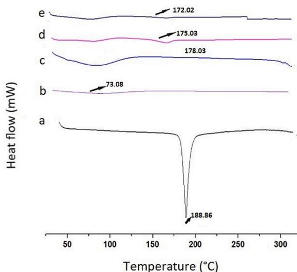
Fig. 5. Thermograms of (a) curcumin (CUR), (b) soluplus, and optimized solid dispersions of CUR with soluplus (c) F1, (d) F2, (e) F3.
