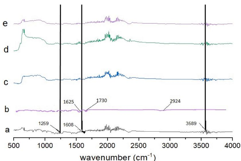
Fig. 2. Fourier transform IR spectra of (a) curcumin (CUR), (b) soluplus, and optimized solid dispersions of CUR with soluplus (c) F1, (d) F2, (e) F3.
