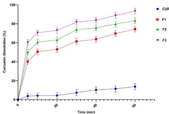
Fig. 6. Dissolution profile of CUR and optimized ternary solid dispersions (F, F2 and F3). Error bars represents standard deviation (N = 3).
