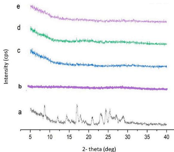
Fig. 3. Diffractograms of (a) curcumin (CUR), (b) soluplus and optimized solid dispersions of CUR with soluplus (c) F1, (d) F2, (e) F3.
