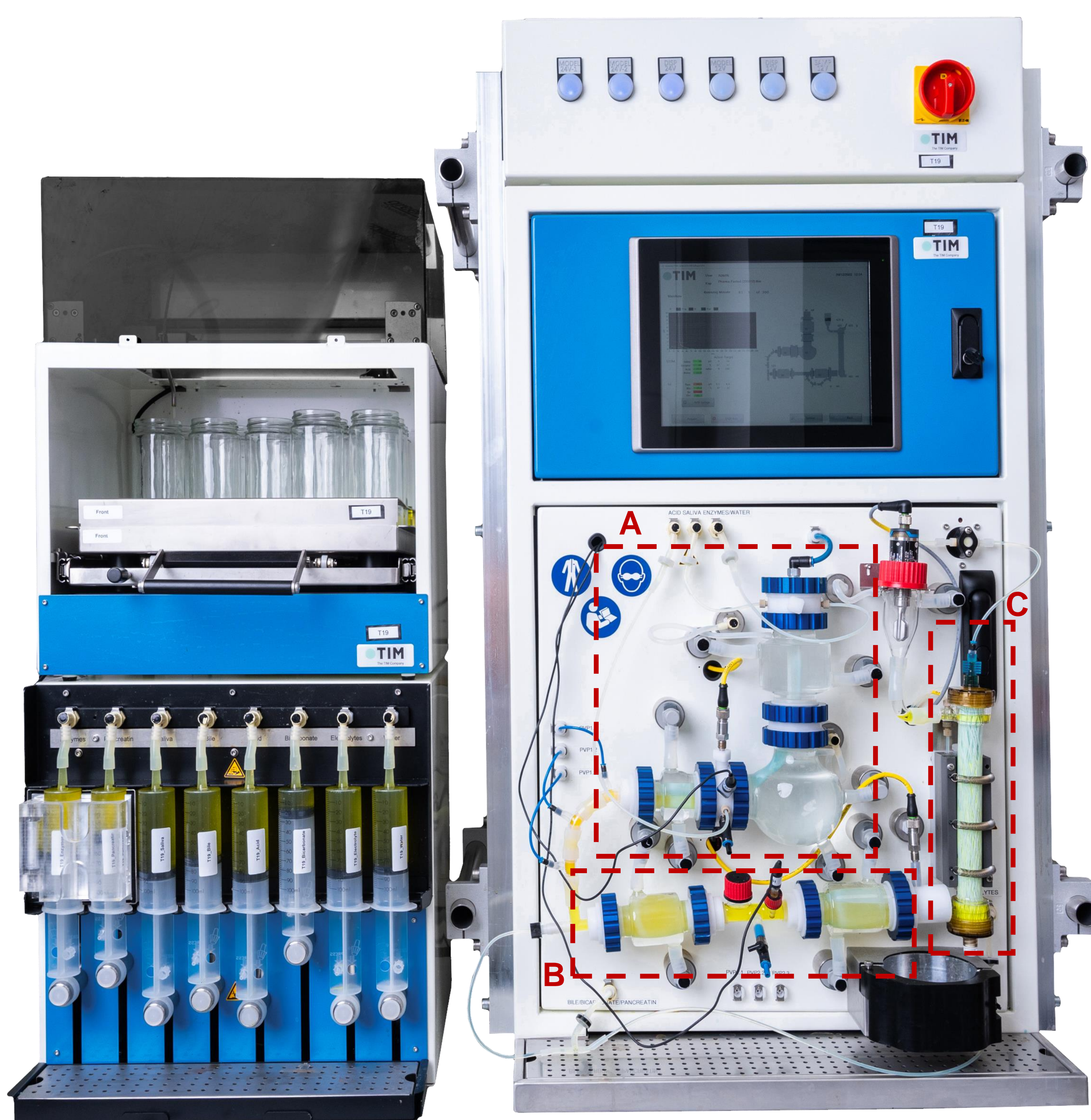
Figure 1. Tiny-TIMsg equipped with the (A) advanced gastric compartment, (B) small intestinal compartment, and (C) filtration system.
