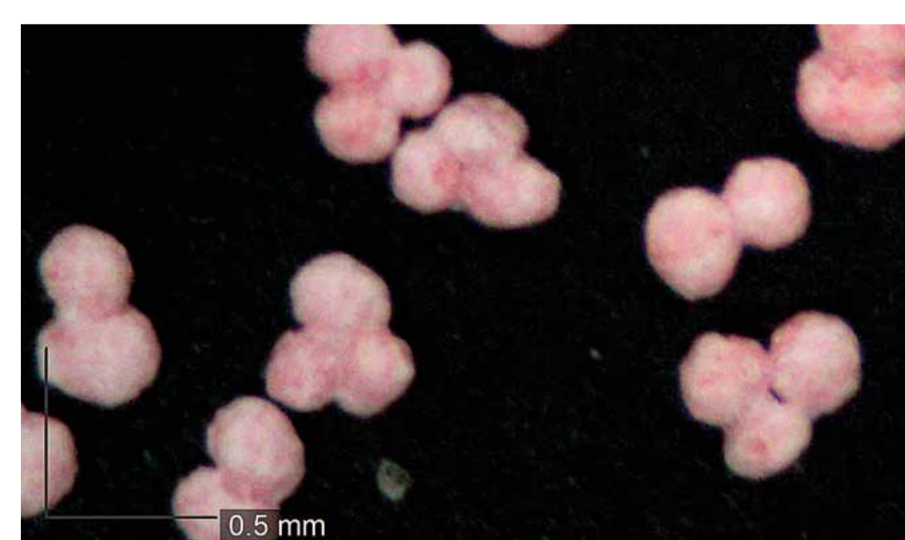
Figure 3: Microscopic image of agglomerated pellets at 75 x magnification
