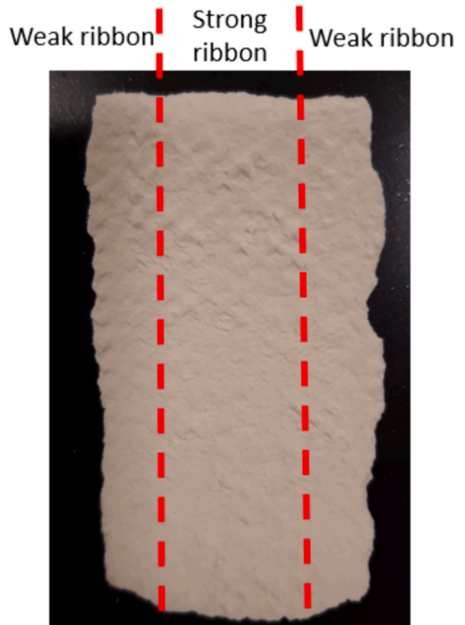
Fig. 7. The middle part of the ribbon is stronger than the two sides of the ribbon as indicated by breakage at the sides.
