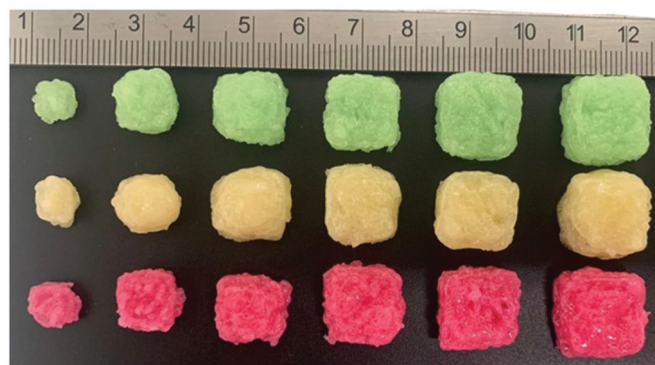
Figure 2. Image of hydrocortisone-loaded chewable printlets containing 1–6 mg, with increasing dose from left to right. The first, second, and third rows correspond to orange-green, banana-yellow and strawberry-red chewable printlets, respectively. Scale in cm.
