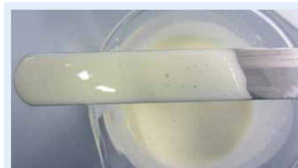
Figure 2. Appearance of the Pickering emulsion containing both retinol palmitate and  $\alpha$ -tocopherol acetate.
