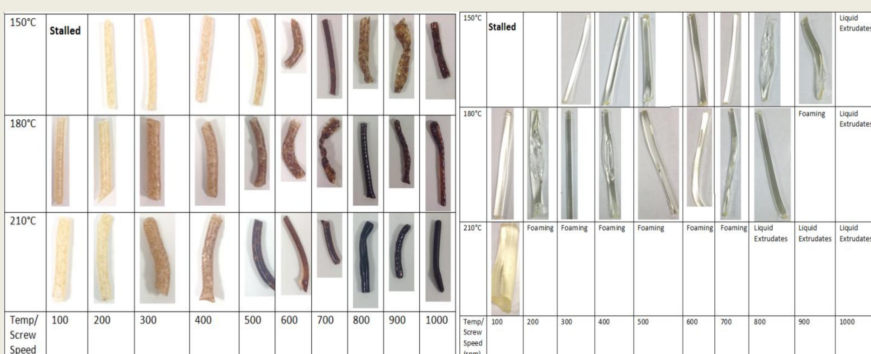
Figure 1: Physical appearance of Affinisol™ 15LV and Plasdone S-630 polymer extrudates
