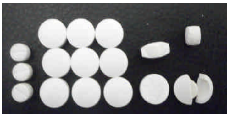
Fig. 11 Oseltamivir Phosphate Tablets after one year storage between 15-25°C From left - core tablets, compression coated tablets and core revealed tablets
